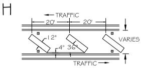
DIAGONAL LINES: I 2" YELLOW OR WHITE LINES INSTALLED AS SHOWN.
