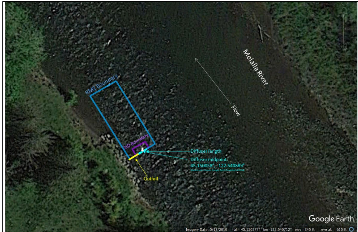
Figure 3-1: Outfall 001 with ZID and RMZ
