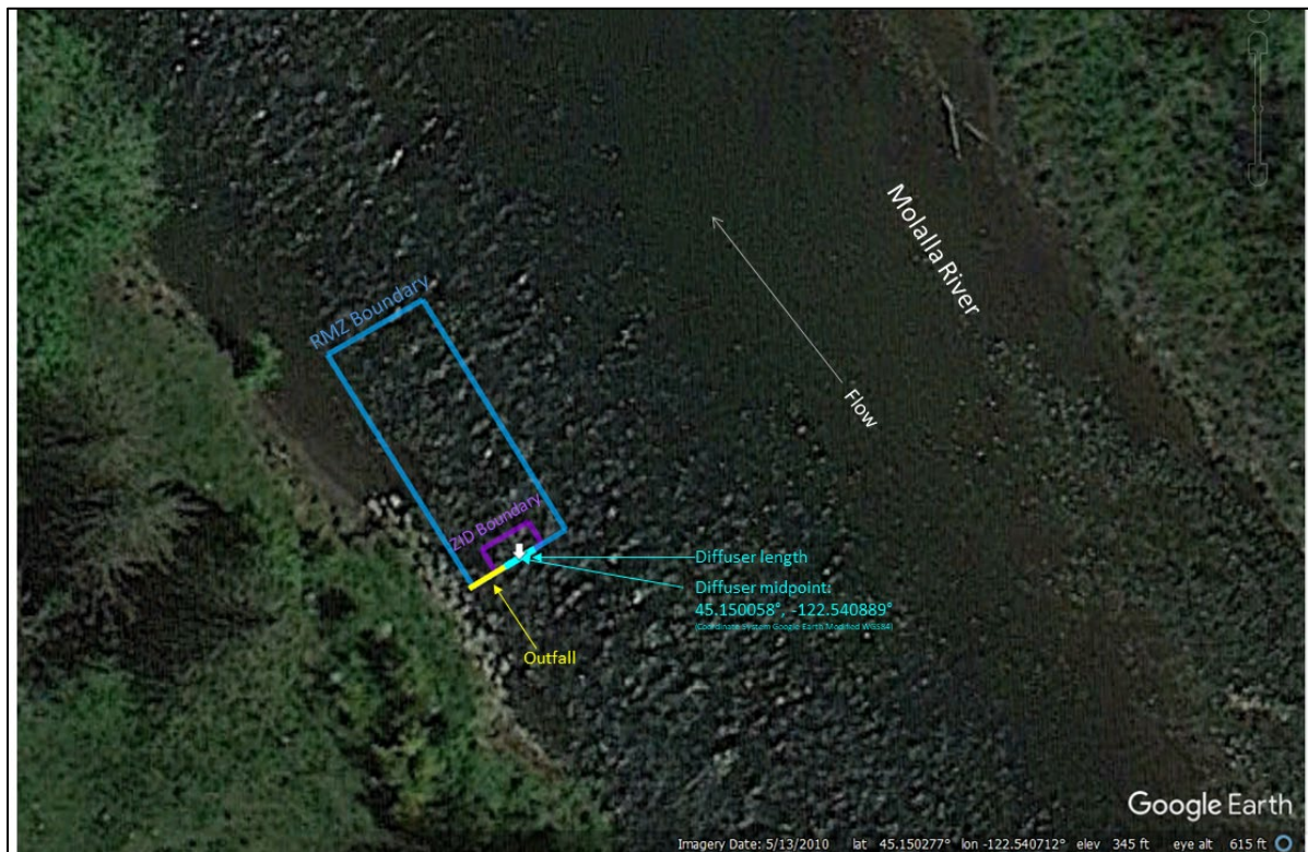
Figure 3-1: Outfall 001 with ZID and RMZ
