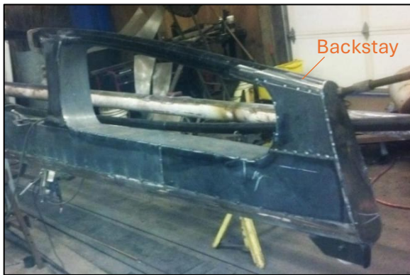
Construction of backstay to create safety pin-like clasp shape at top of each pole
