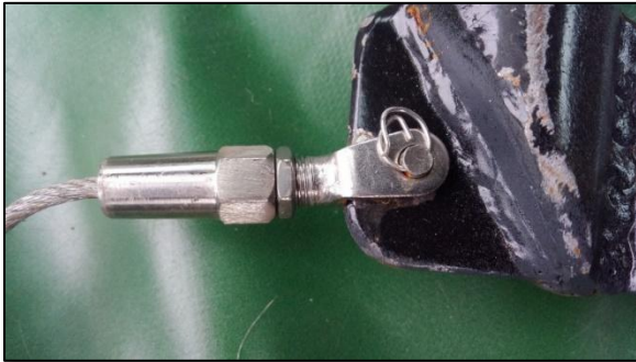
Hoisting wire is 3/32-inch 7 x 9 steel cable
