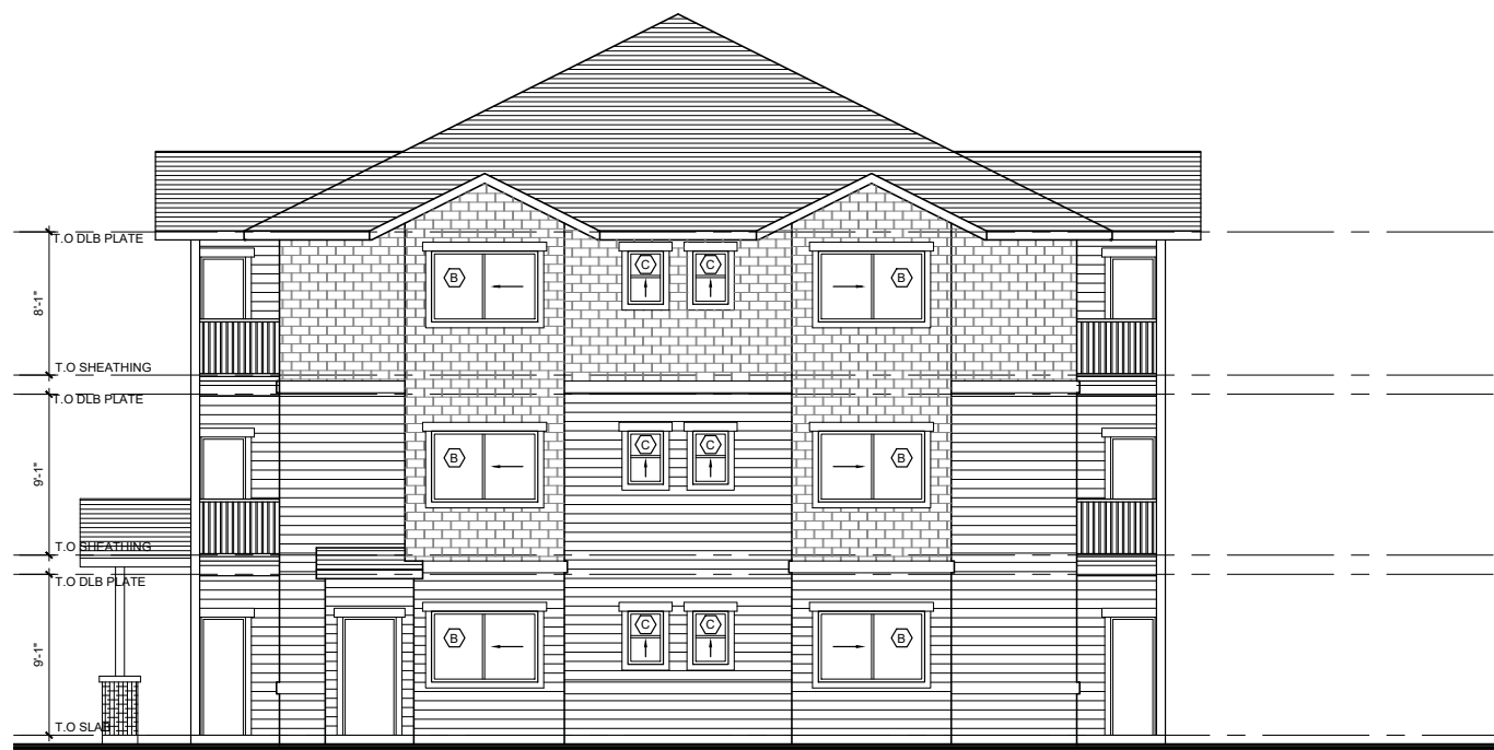
2 BUILDING ELEVATION A203 3/16" = 1'-0"
