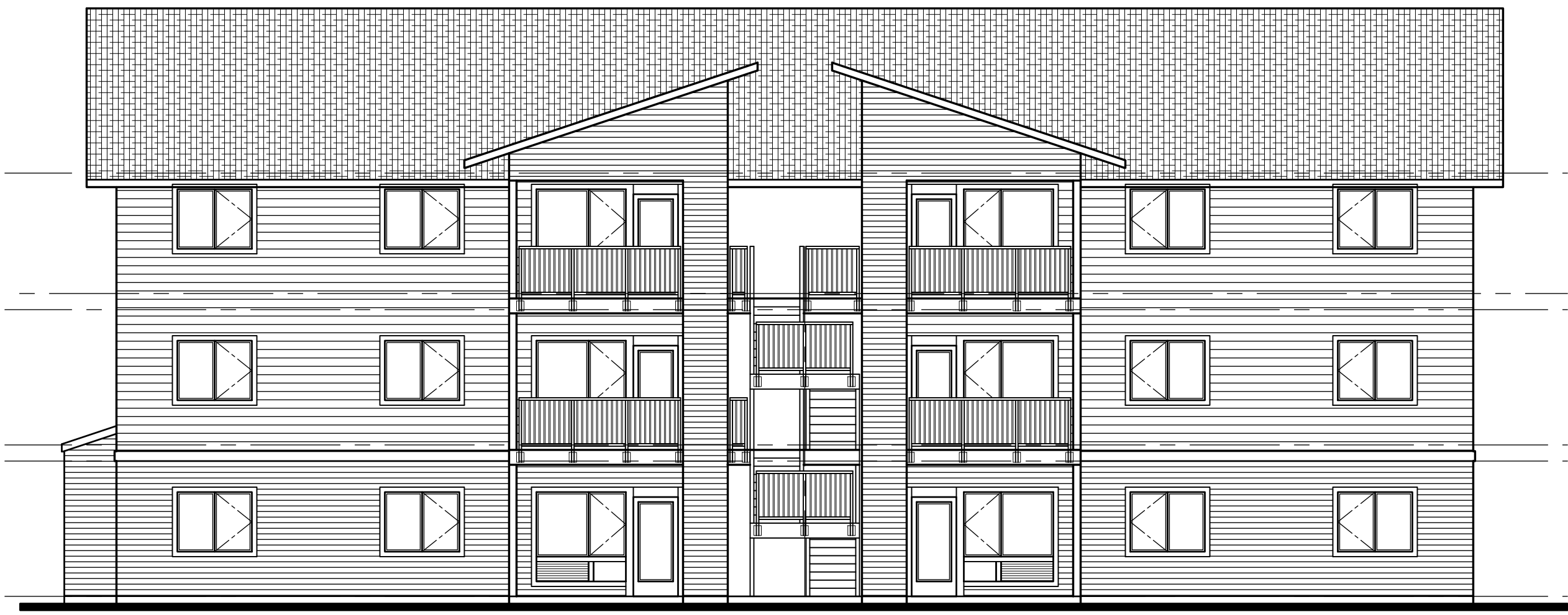
4 EAST ELEVATION - BUILDING B 1/8" = 1'-0"
