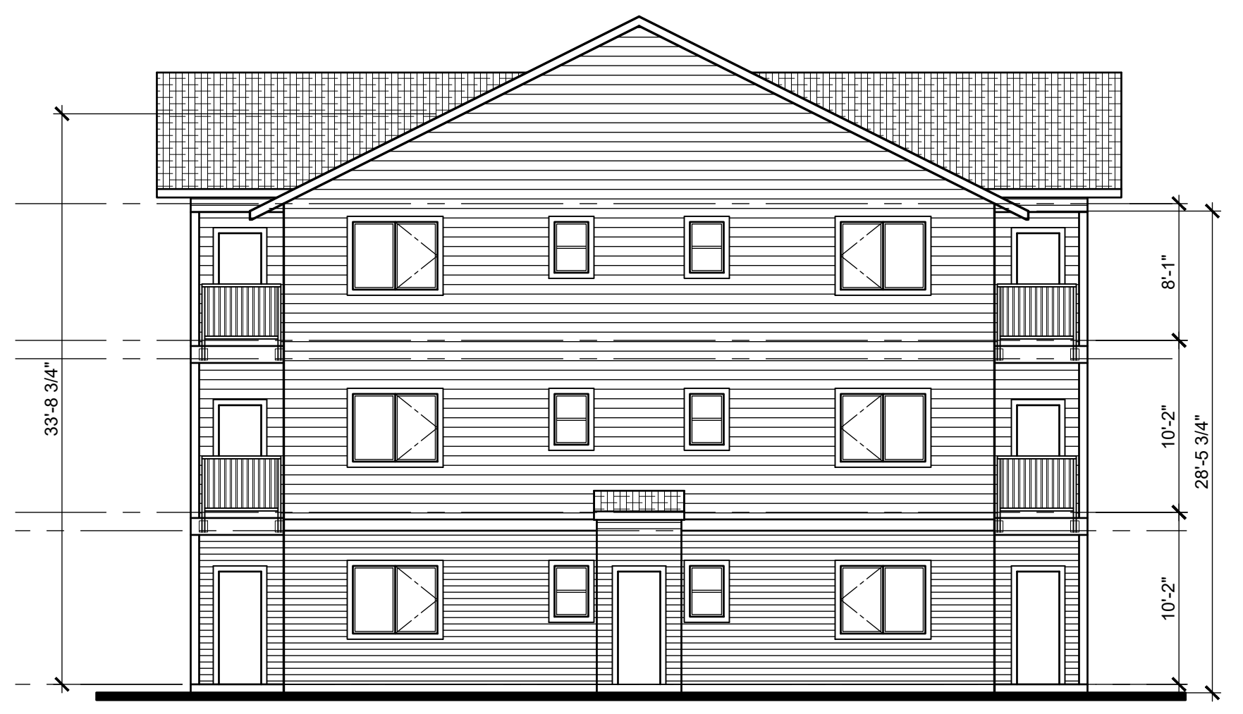
2 SOUTH ELEVATION - BUILDING B 1/8" = 1'-0"
