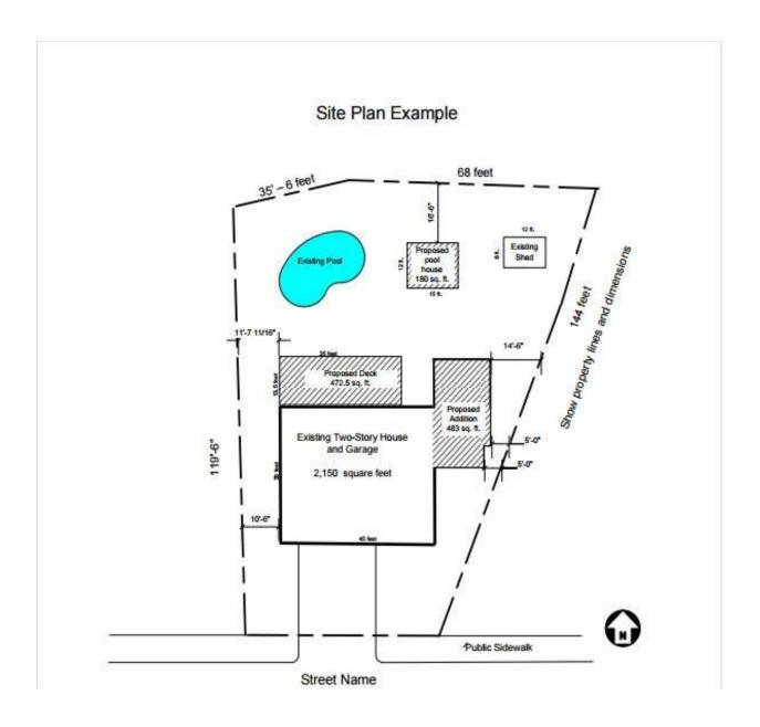
This sample site plan does not include every element required in the Site Plan Checklist but is an example of an acceptable format to use. This may be hand drawn or computer generated.
