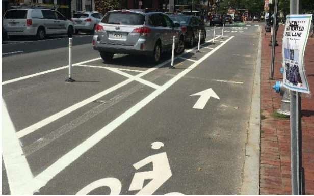
Example of One-way Parking Protected Bike Lane
