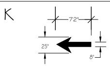
BICYCLE LANE ARROW: SEE ODOT BIKE LANE STANDARDS. USE PREFORMED THERMOPLASTIC PAVEMENT MARKING MATERIAL.
