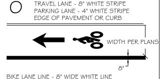
BICYCLE LANE MARKING: SEE ODOT BIKE LANE STANDARDS. USE PREFORMED THERMOPLASTIC PAVEMENT MARKING MATERIAL.
