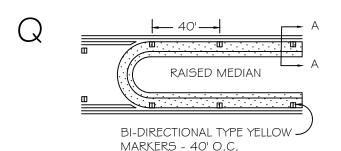
RAISED MEDIAN STRIPE: 4" YELLOW LINE WITH TYPE I BI-DIRECTIONAL YELLOW RAISED PAVEMENT MARKERS AT 40' O.C.
