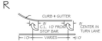
RIGHT TURN LANE MARKINGS: SEE MUTCD AND ODOT STANDARD DRAWING TM530 FOR DETAILS. ARROWS SHALL BE THERMOPLASTIC PAVEMENT MARKING MATERIAL.
