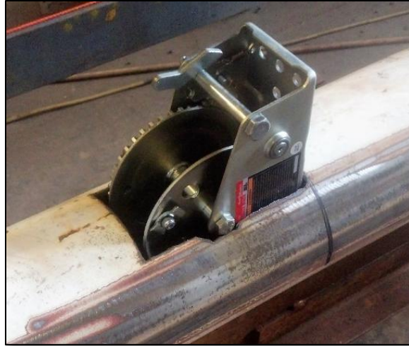
Hoisting winch has a 1500-pound linear pull capacity
