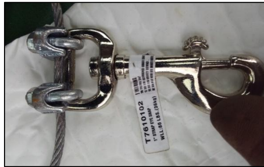
Hoisting wire is 3/32-inch 7 x 9 steel cable
