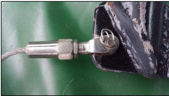
Hoisting wire is 3/32-inch 7 x 9 steel cable
